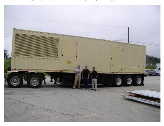
70 dB(A) @ 1 mtr enclosure on a 2000 kWe gen set on a UL142 3000 gallon tank.
