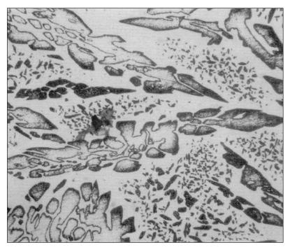
This photo is an optical microscopic view of WCD4<sup>TM</sup> at x250 magnification. The microstructure consists of primary and secondary austenite grains embedded into the ferritic matrix.
