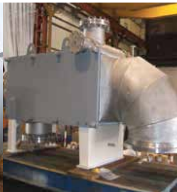
Condenser on methionine reactor
